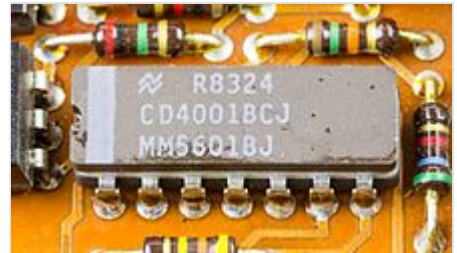
CD4001B quad 2-input NOR gate in DIP-14 package, manufactured by National Semiconductor in 1983
