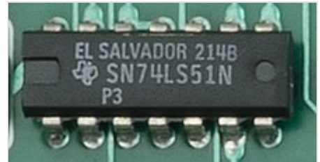
TI SN74LS51 in DIP-14 package
