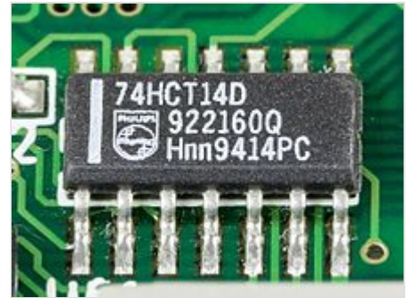
Philips 74HCT14D, a hex inverting Schmitt trigger
